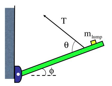
2.) A beam of length "L" is pinned at an angle θ to a wall (see sketch). Tension in a rope "3L/4" from the pin keeps it in equilibrium. There is a massive lump a distance "5L/6" units up the beam. What is known is:
